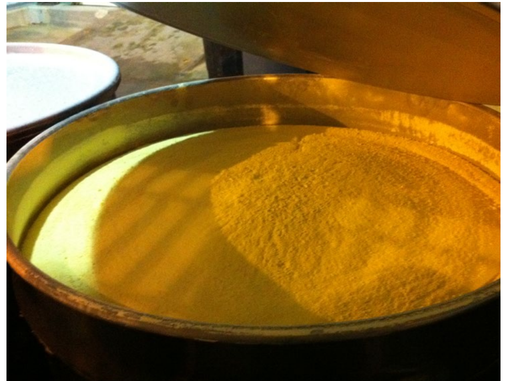
Image: Yellowcake is the raw material for manufacturing nuclear fuel. Source Uranium Energy Corp, US
