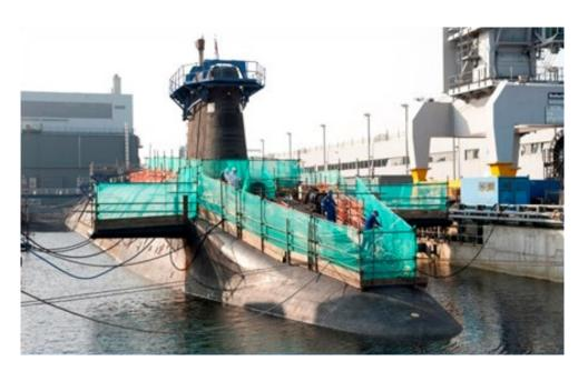
Image: The nuclear-powered submarine HMS Vengeance at Devonport dockyard during a periodic refit and refuelling operation. Source - Ministry of Defence
