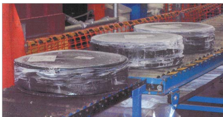
Drums of LLW after supercompaction
