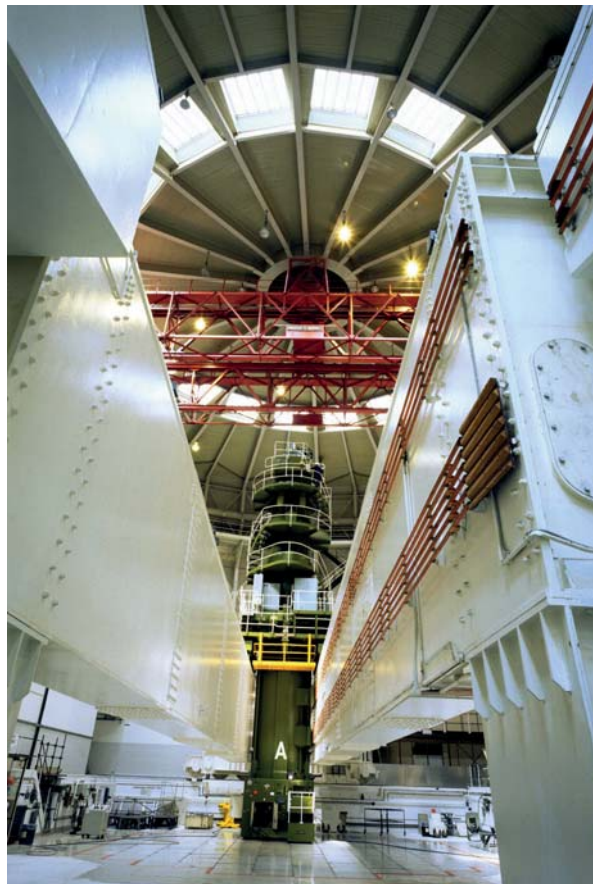
Figure 4.3: View across top of Oldbury reactor showing machine for changing Magnox fuel elements
