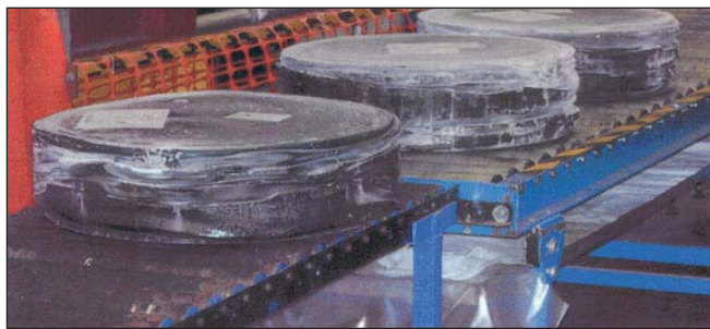
Drums of LLW after supercompaction
