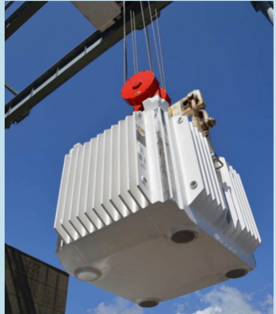
Image: A reactor may contain over 50,000 fuel assemblies that all need to be removed from the site during defuelling. These will be transported in special containers like the one shown here
