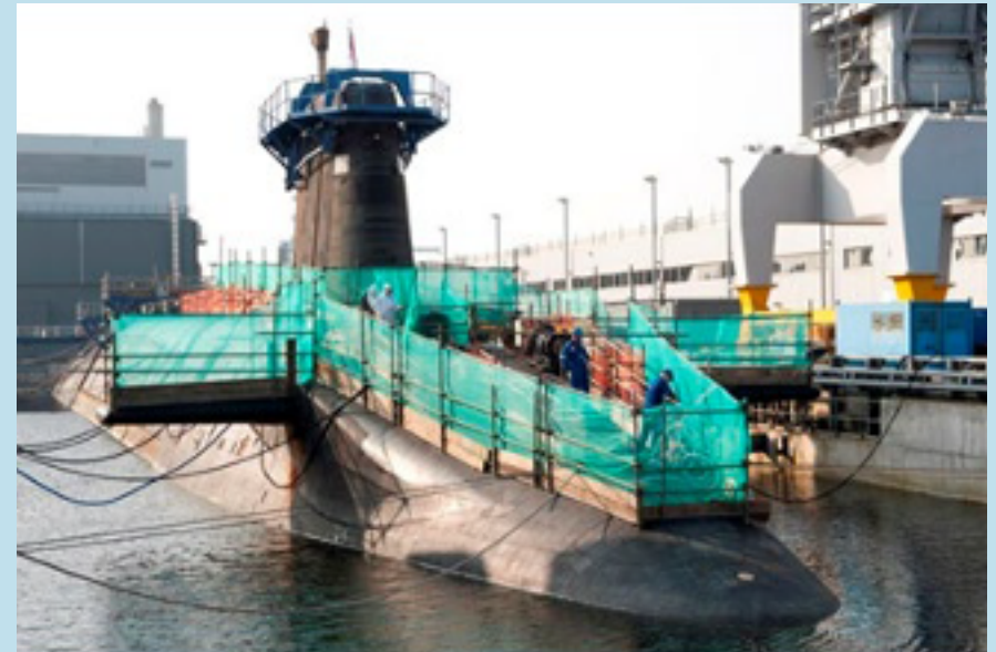
Image: The nuclear-powered submarine HMS Vengeance at Devonport dockyard during a periodic refit and refuelling operation. Source - Ministry of Defence
