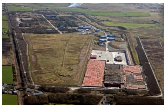
Aerial view of the LLWR showing vaults of disposed low activity waste
